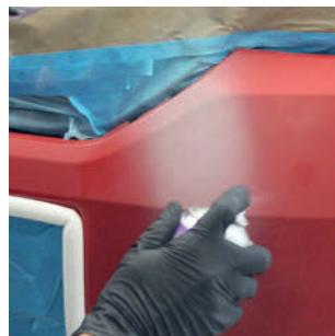
Use the UV Cleaner to remove the tacky residue. Sand the entire surface.
