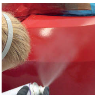
Apply UV Spot Blender Thinner into transition zone and allow 1 min flash off time.
