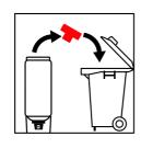
To ensure that it is immediately apparent that the hardener has been triggered, the red button should not be put back into the can cap after the triggering process, but should be disposed of immediately.
