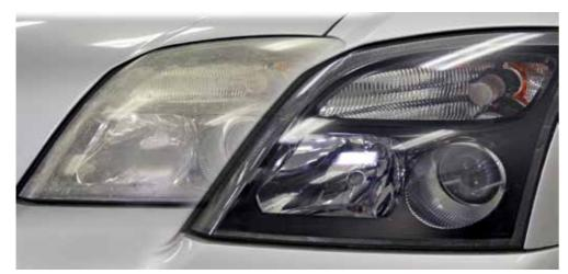
Before: Matting/yellowing, slight superficial scratches to the coating. After: Once dry, surface is permanently sealed. If necessary, can be wet sanded and polished.
