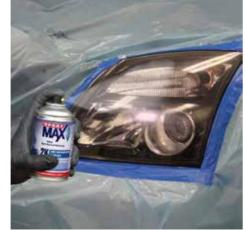
Apply a very thin (misty) layer of clearcoat first, directly followed by a continous, film-forming spray pass.
