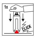
Press can down with even pressure. Listen for cracking sound. Press only once.
